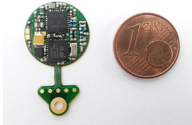
Fig. 1. Assembled PCB in comparison to a 1 Euro Cent coin. The flag gets folded around the battery for connecting the plus pole.
