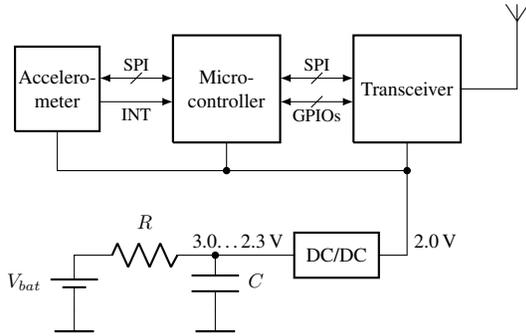
Fig. 2. Block diagram of the voltage supply and interconnections.
