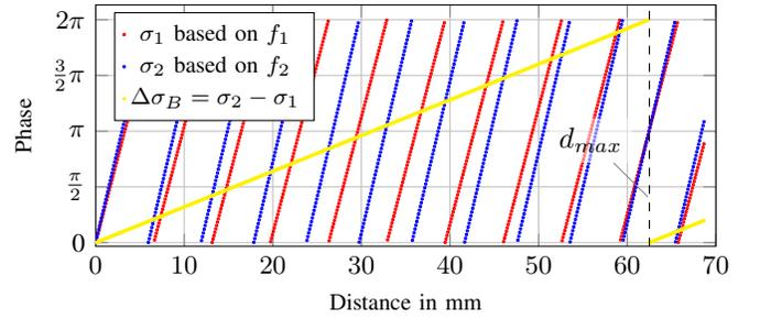
Fig. 2. Phase responses for two different frequencies (blue, red) at the same distance and corresponding beat frequency phase (yellow).
