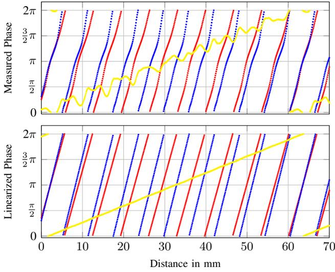
Fig. 3. Raw measured phases (top) in RAD with the dual tone system for a frequency spacing of 2.4 GHz and linearized phases of the same signal (bottom).
