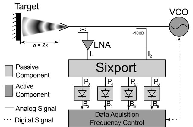
Fig. 1. Overview of a Six-Port radar front-end for distance measurements.
