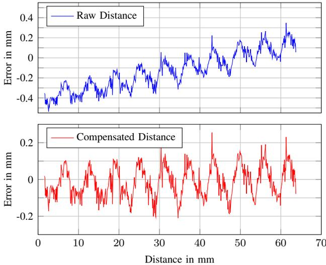
Fig. 4. Calculated distance error at 2.4 GHz frequency spacing without compensation (top) and compensated for the beat frequency shift (bottom).
