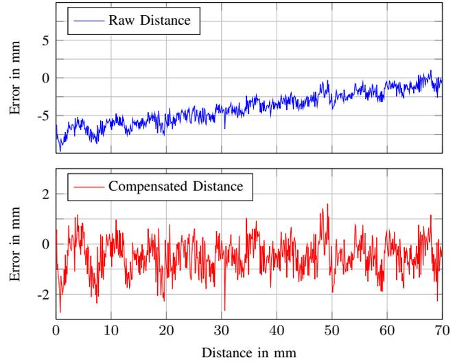
Fig. 5. Calculated distance error at 250 MHz frequency spacing without compensation (top) and compensated for the beat frequency shift (bottom).
