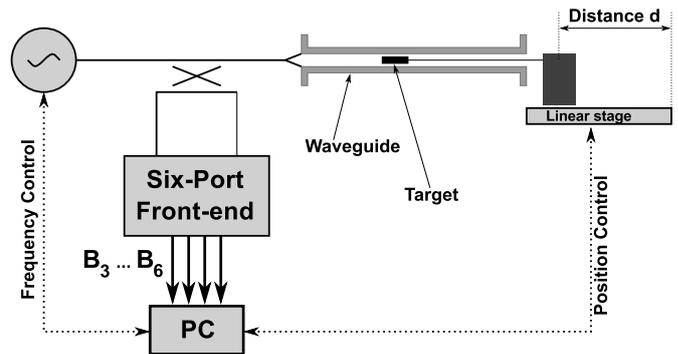
Fig. 1. Measurement setup for waveguide based distance evaluation.
