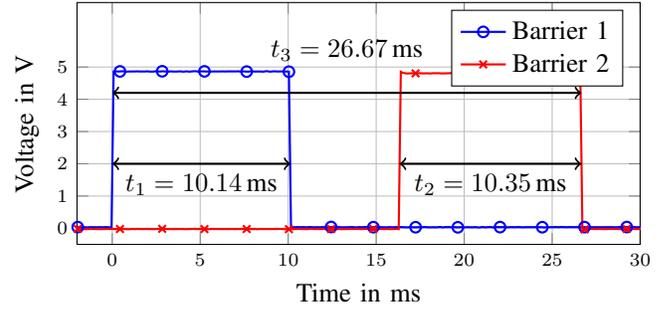
Fig. 5. Interruption event of both laser barriers measured at the oscilloscope
