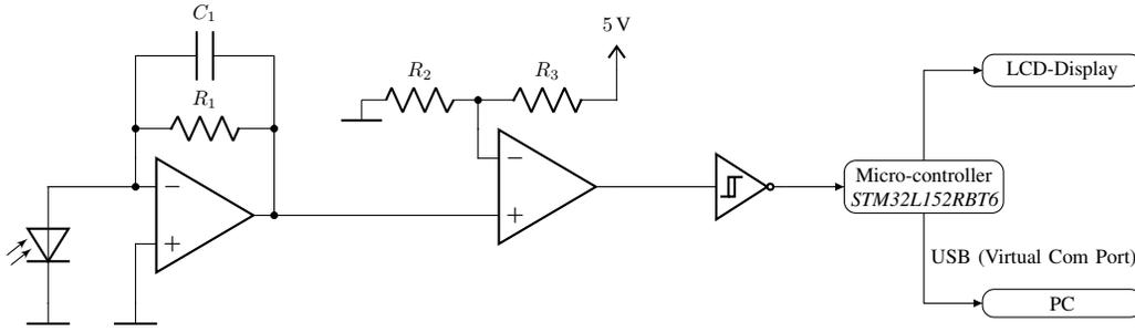
Fig. 2. Read out circuitry for photo diode
