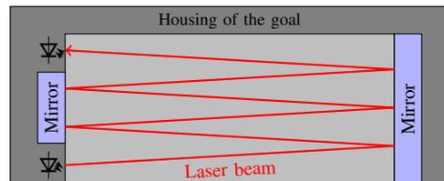
Fig. 3. Laser fence to enhance detection range using mirrors
