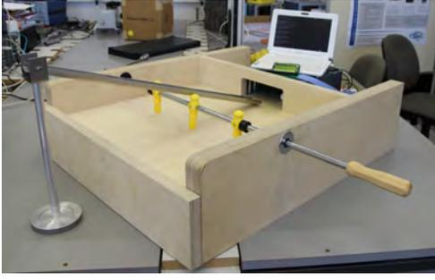
Fig. 4. Demonstrator setup with well-defined inclined plane for accuracy measurements
