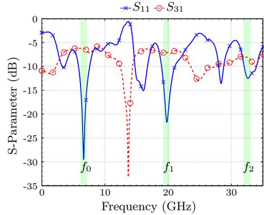
Figure 4: Simulated reflection and transmission coefficients of the Six-Port junction over the entire frequency bandwidth.
