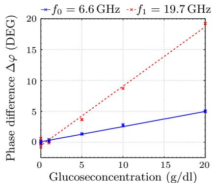
Figure 7: Measured phase difference of the sensor's transmission coefficient for varying glucose concentrations.
