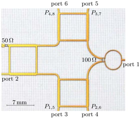
Figure 3: Photo of the Six-Port network realized in microstrip transmission line technology on a dielectric substrate (reflection: indexes 1 to 4; transmission: indexes 5 to 8).
