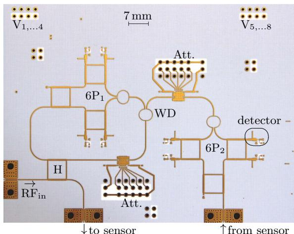
Figure 5: Photo of the designed multiband VNA.
