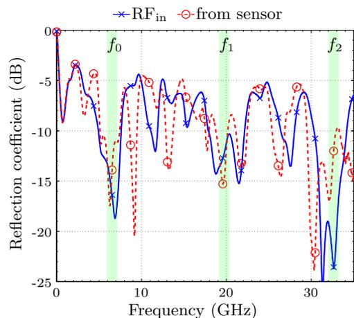
Figure 6: Measured reflection coefficients of the VNA's input ports.
