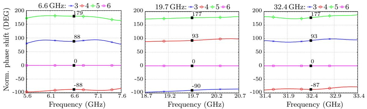
Figure 8: Measured relative phase shifts at the output ports 3 to 6 of the Six-Port network normalized to a phase shift of 0 DEG at port 6
