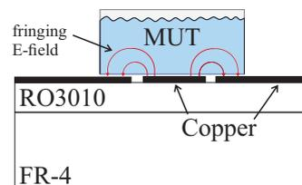
Figure 1: Schematic cross section of the utilized coplanar waveguide sensor.
