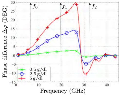
Figure 2: Simulated phase difference of the sensor's transmission coefficient due to glucose concentration variation.
