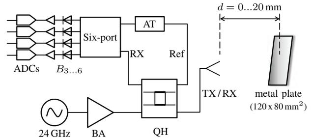
Fig. 1. Block diagram of the system (BA: buffer amplifier, QH: quadrature hybrid, AT: attenuator).
