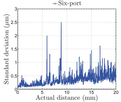
Fig. 6. Standard deviation of the measurement results over the distance between target and antenna.
