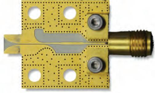
Fig. 2. Photo of slot-line antenna with transition to microstrip transmission line.
