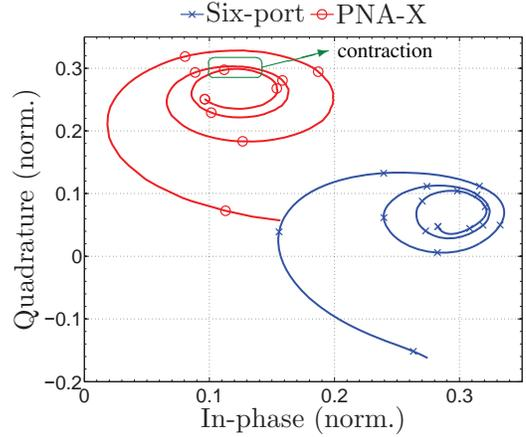
Fig. 3. Measured reflection of the antenna at 24 GHz for target positions from 0 mm to 20 mm.
