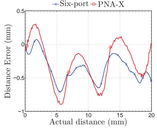
Fig. 5. Error curve comparison of the near field measurement by the proposed Six-port network and the commercial VNA *PNA-X*
