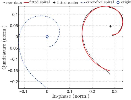
Fig. 4. Measured (black), fitted (red), and calibrated (blue) spiral of measured Six-port data for displacement from 0 to 6.6 mm.
