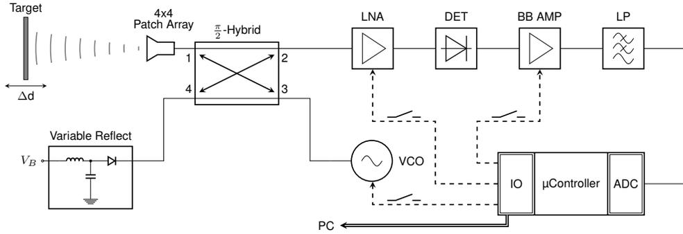
Fig. 1. System concept of the proposed low-power radar system.
