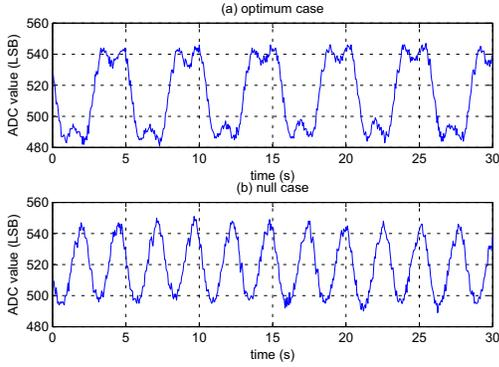
Fig. 4. Raw ADC measurement results without any further processing for a mechanical target movement with  $\Delta d = 5$  mm peak-peak and an oscillation frequency of 0.2 Hz, in the distance  $d = 2$  m for (a) the optimum case (b) the null case.
