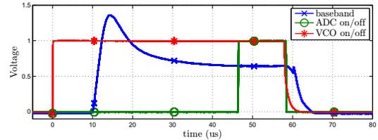
Fig. 3. Measured baseband voltage and active timing signals of the VCO and ADC.
