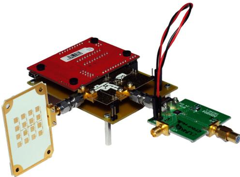
Fig. 2. Photo of the developed radar system prototype.
