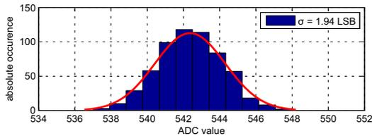
Fig. 5. Repeatability of the measurements in an empty room. In total 600 measurements were performed within 30 seconds.
