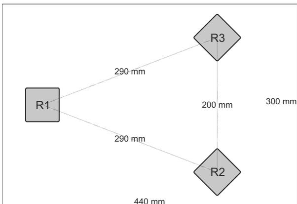
Fig. 1. Scheme of the receiver board
