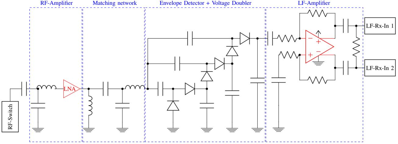
Fig. 3. Signal processing circuit for the wake-up-receiver with LNA, matching, envelope detection, voltage doubling and LF-amplification
