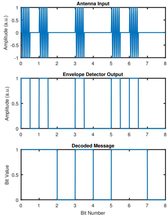
Fig. 2. Simulation of creating an LF-OOK-signal from higher frequency OOK-bursts
