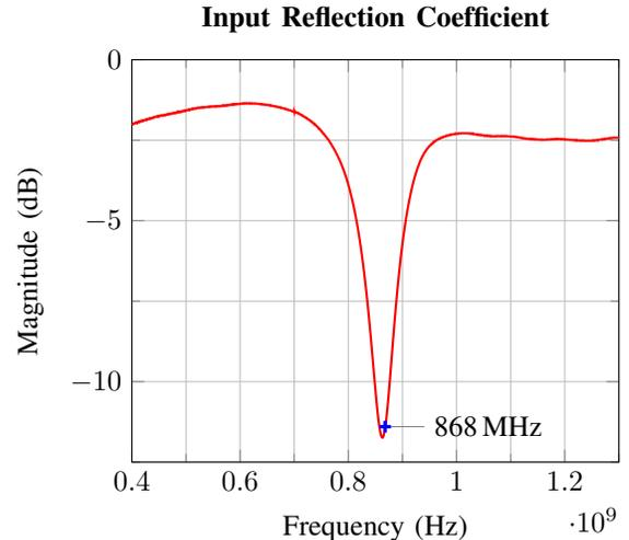
Fig. 4. Input reflection coefficient  $S_{11}$  of the Rx-path
