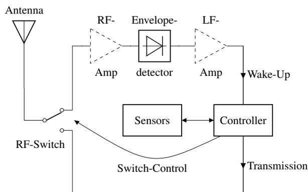
Fig. 1. Block diagram of the sensor node's functional units
