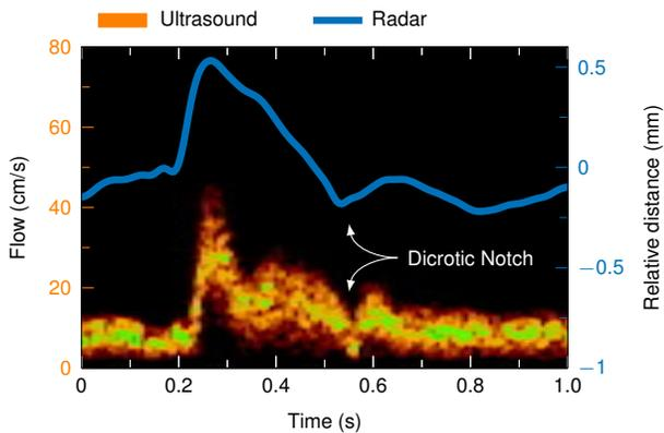
Fig. 4. A single heartbeat from a synchronous measurement using radar and ultrasound. Both signals show a high similarity and feature the same characteristics.
