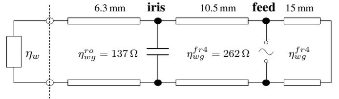
Fig. 6. Equivalent circuit diagram of the proposed antenna
