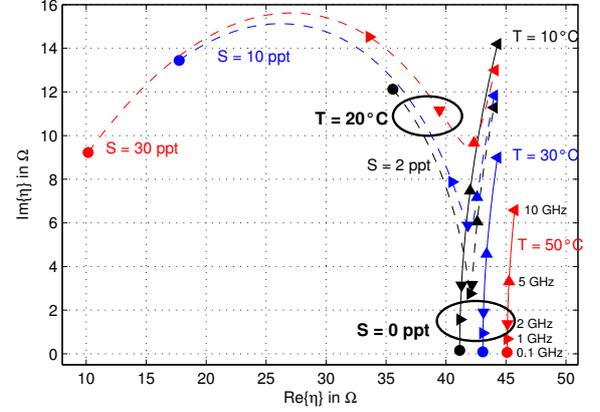
Fig. 3. Real and imaginary part of the intrinsic impedance of water between 0.1–10 GHz for different temperatures (solid lines) and salinities (dashed lines). Markers indicate the frequency (see labels in the bottom right-hand corner).
