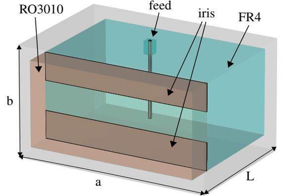
Fig. 5. Simulation model of the proposed antenna
