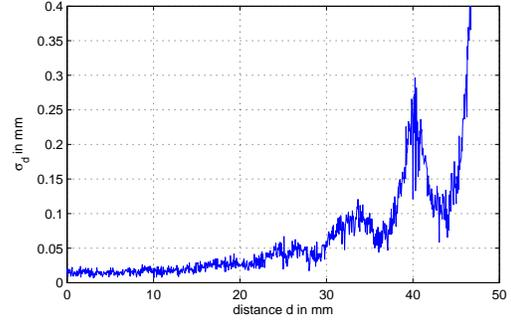
Fig. 5. Standard deviation  $\sigma_d$  of the dist. meas. error (10 sweeps)
