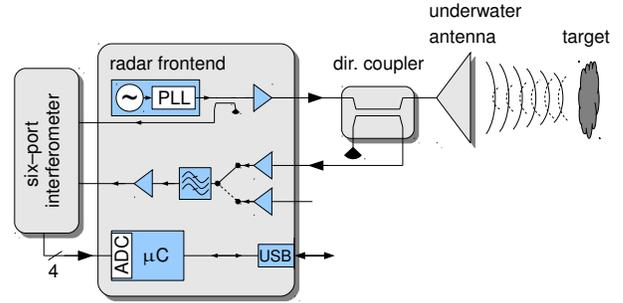
Fig. 2. Block diagram of the underwater distance meas. system
