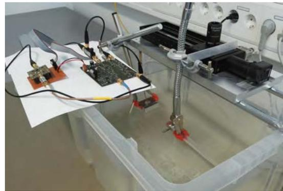
Fig. 3. Measurement setup showing radar frontend, six-port interferometer, directional coupler, underwater antenna and target mounted on a linear stage
