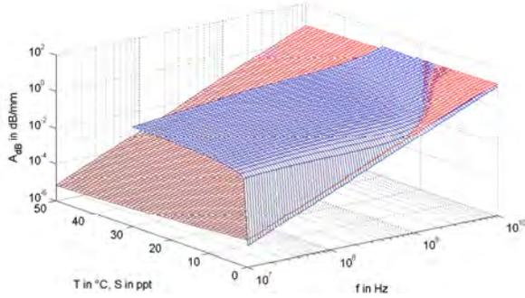
Fig. 1. Attenuation of a plane EM wave in water for  $f = 0.01 - 10$  GHz. The red surface shows the dependence on temperature with  $S = 0$ . The blue surface shows the dependence on salinity at  $T = 20^\circ$ .
