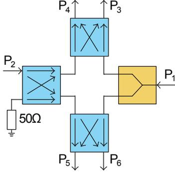
Fig. 1. Circuit schematic of the Six-Port network.
