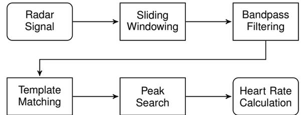
Fig. 3. Flow chart of the heartbeat analysis by cross-correlation based template matching.
