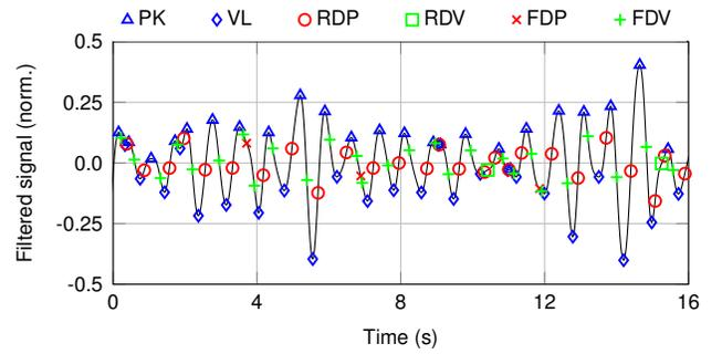
Fig. 3. Detected features in the filtered radar signal.
