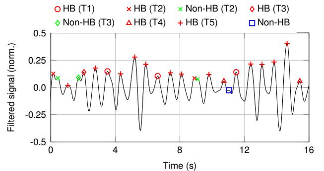
Fig. 4. Detected heartbeat types in the filtered radar signal.
