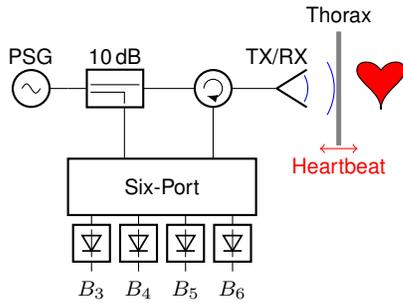
Fig. 2. Block diagram of the Six-Port sensor.
